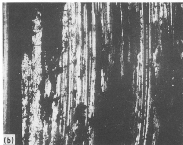
Figure 8 Optical microphotographs (X1000) of cobalt (a) before and (b) after the wear test.
